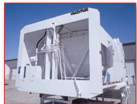
Body-mounted hydraulic reservoir and filter assembly
